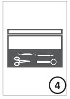
Disassemble the instruments and place them in the solution. Make sure that the solution completely covers the instruments. Close the lid of the bath.
