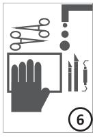
Remove the instruments from the solution and rinse with water of at least drinking quality, and dry them. If necessary, repeat the cleaning process and brush the instruments with a suitable brush.
