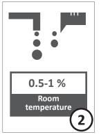
Fill the instrument bath Move the strainer with water (at room temperature). Add Actoclean® Flussig according to the recommended concentration of use.
